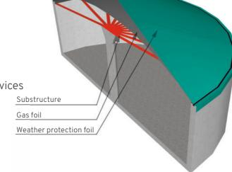
Our double membrane gas storage system does not necessarily have to be installed on a tank. A concrete surface or a ring foundation made of concrete can be used as a substrate, for which we supply a suitable ground seal. This also has the advantage of being able to easily achieve higher operating pressures. We use our stainless steel flat section for fastening. This design also allows you to choose between different shapes (round, square, oval) and heights, depending on the required volume.
